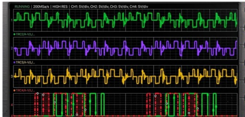
Fig. 12: Gate control signal overlaps and waveform switching collisions under VPWL coordination
