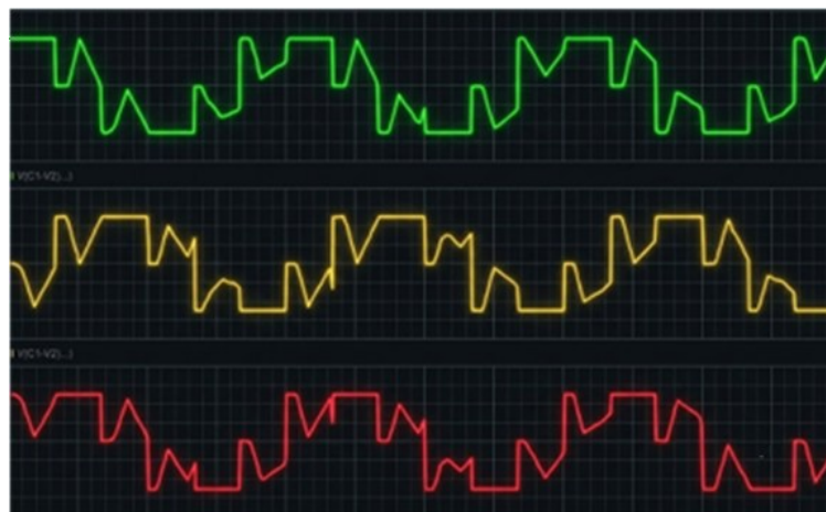
Fig. 7 Geometric collapse of line-to-line voltage ( V_{ab} ) into a triangular profile under 120^\circ conduction mode for Case 4.
