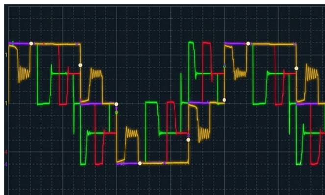
Fig. 10: Line voltage characteristics under pulse width (6 ms – 12 ms) with 100 mH
