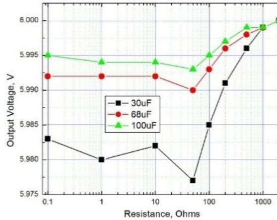
Fig. 6. Variation of the Output Voltage with Capacitance
