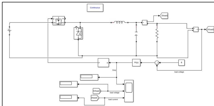
Fig.5. Buck converter schematic diagram with the PWM
