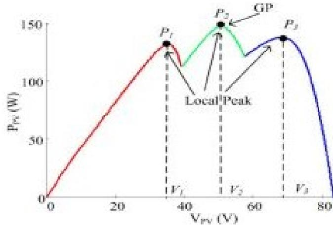
Fig. 9. PV curve for an entire array [5]
