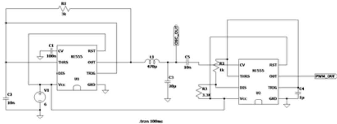
Fig. 3. Schematic of a dual 555 timer
