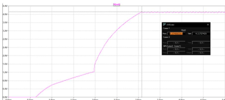
Fig. 9. Output voltage for the circuit of LTC3105
