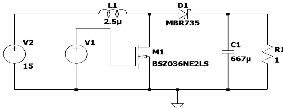
**Fig. 2.** Schematic diagram of the Booster circuit
