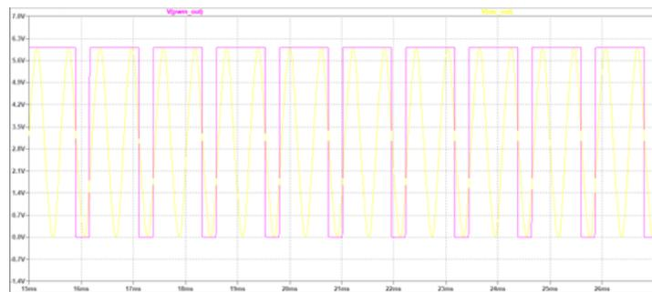
Fig. 8. Output voltage of the 555 timers
